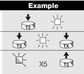
Note: if there are other transmitters to erase repeat the steps for each transmitter. If a transmitter is memorised in mode II, each memorised key must be erased.
