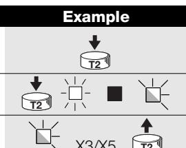
Note: During the erasing procedure the "radio LED" will flash rapidly: 5 flashes will signal that the procedure has been completed.
